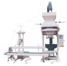
Bag filling Machine (For 10Kg to 50 Kg)
